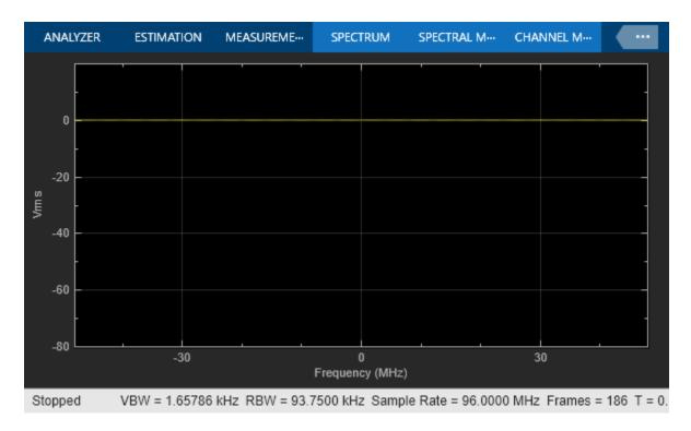
The Spectrum Analyzer block now shows a sample rate of 96 MHz, which is 1.5 times the previous sample rate, as expected.
