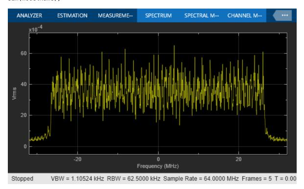
The Spectrum Analyzer block inherits the **Waveform sample rate (Fs)** parameter, which is 64 MHz. close\_system(modelName);
