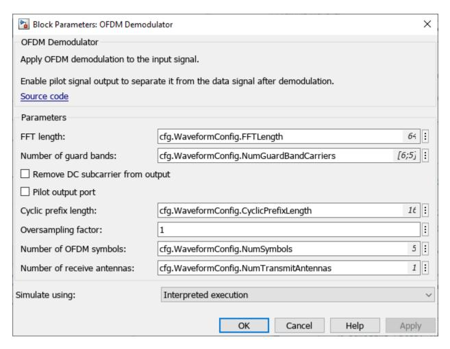
Because the OFDM Demodulator block requires the entire OFDM waveform for demodulation, set the **Samples per frame** parameter in the exported block to cfg.WaveformLength. Simulate the model.
