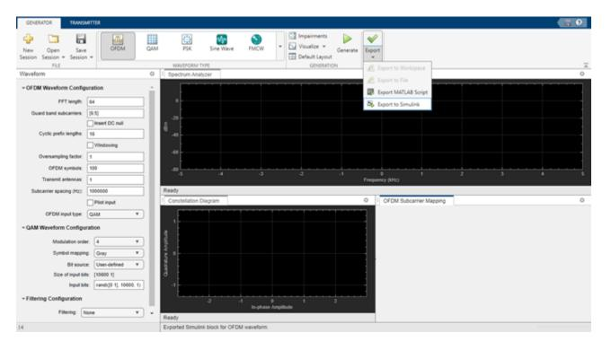
The **Export to Simulink** option creates a Simulink block, which outputs the selected waveform when you run the Simulink model. The block is exported to a new model if no open models exist.
