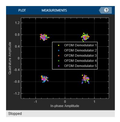
After demodulating the OFDM waveform by using the OFDM Demodulator block, the Constellation Diagram block displays the resulting QAM symbols.
