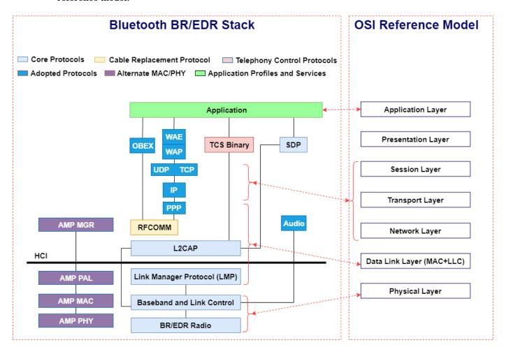
The mapping of BR/EDR stack to the OSI reference model is as shown below:
