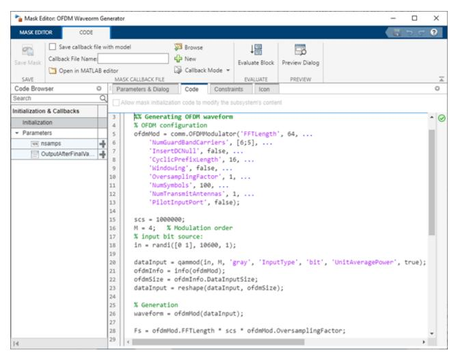
Use the MATLAB code that is available in the **Code** tab to update the parameters of your choice. For example, set the subcarrier spacing, scs, to 1,500,000 Hz.
